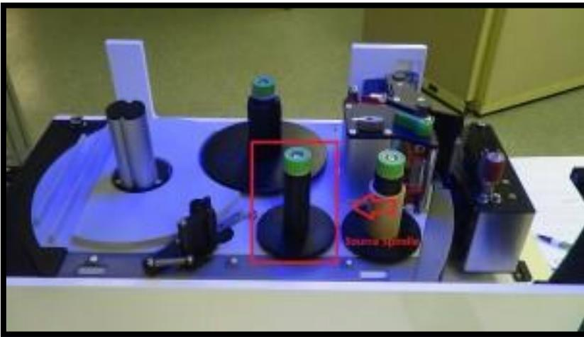
**Step 3.** Attach the ribbon to the take up core so it can wind counterclockwise. Use a label to attach it if necessary.
