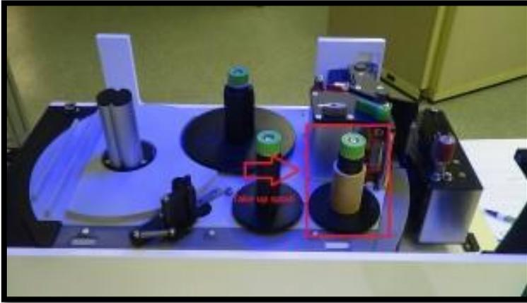
**Step 5.** Turn the ribbon take up spool counterclockwise to wind the ribbon through the system and ensure there are no wrinkles as it moves through the head.
