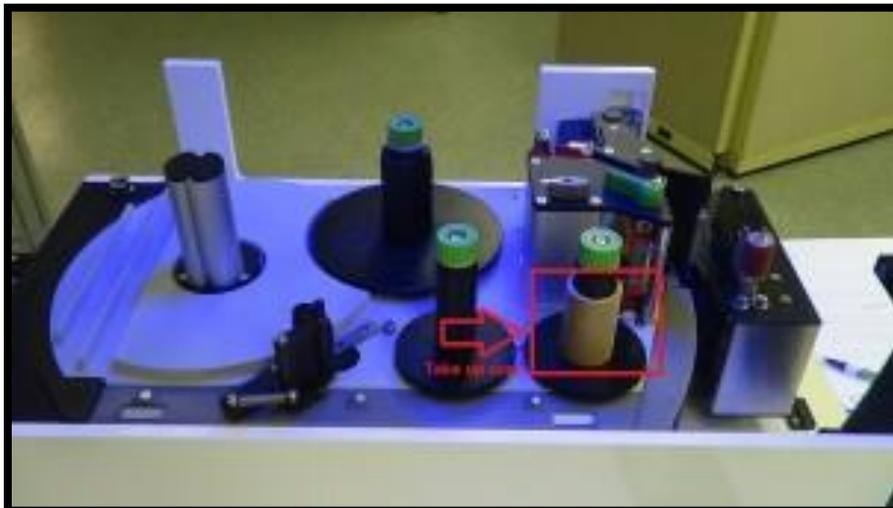
**Step 4.** Place the core on the take up spool. Turn the green knobs on the source and take up spindles counterclockwise to lock the ribbon cores. Failure to do this will result in an “out of ribbon” error.
